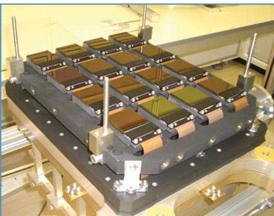
Figure 3. 64-megapixel FPA composed of sixteen SWIR 2Kx2K FPA modules
