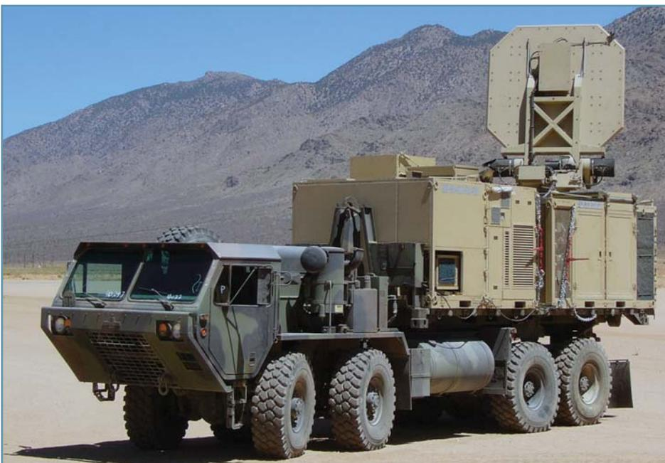
Figure 3. Raytheon’s ruggedized Active Denial System 2 includes a fuel supply and generator for long-term operation in remote areas.
