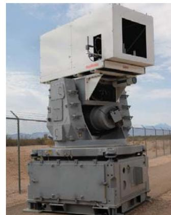
*Figure 1. This LADS prototype combines proven Phalanx weapon system capabilities with commercially available laser and optical components.*
