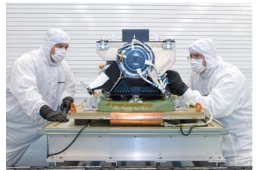
Raytheon sensor designed to promote understanding of global warming passed vibration testing
