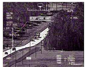
Infrared, Ultranarrow FOV (2.4 nmi)
