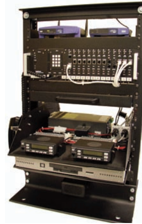
Photo caption: Left: A typical ACU-1000 fixed site configuration. Top Right: ACU controller software. Bottom Right: WAIS controller software.
