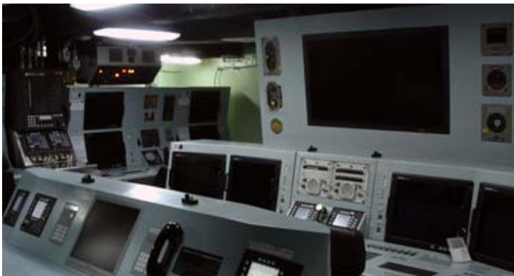
Modern high-resolution, color consoles enable the viewing and tracking of targets from various radars with mapping and expanded detection, as well as engagement and symbol capabilities in user-friendly, customizable window views.
