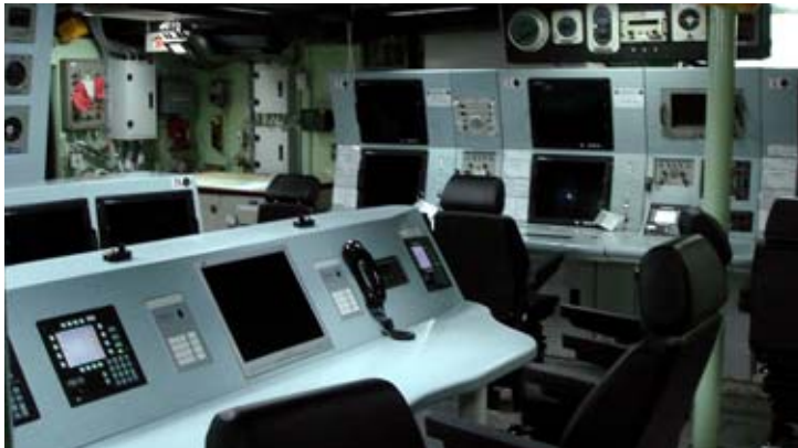
Modern high-resolution, color consoles enable the viewing and tracking of targets from various radars with mapping and expanded detection, as well as engagement and symbol capabilities in user-friendly, customizable window views.
