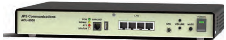
Photo caption: Raytheon's ACU-5000 can be used as a gateway for local interoperability
