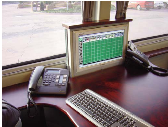
ACU Controller software in use in Turkey mobile communications vehicle
